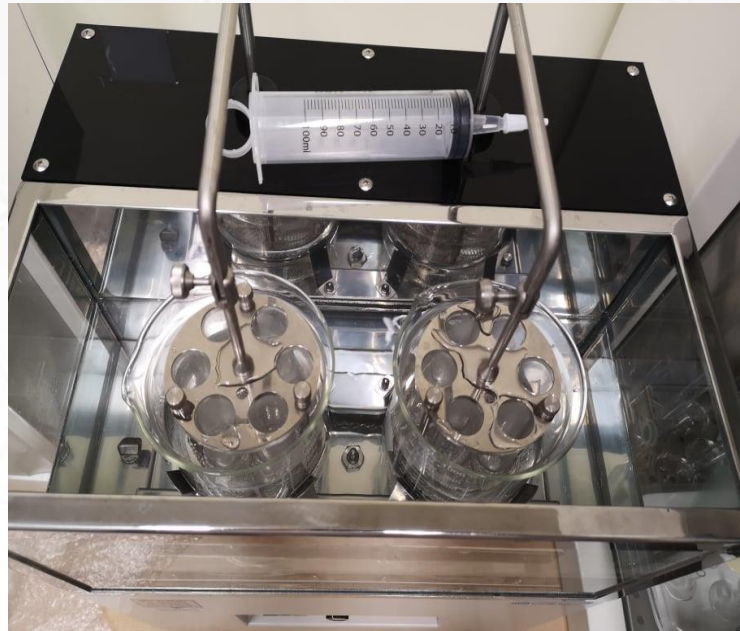
Figure 6,7. The device performs a disintegration test at MRC Scientific Instruments.
