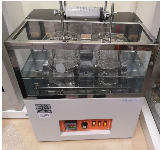
Figure 6,7. The device performs a disintegration test at MRC Scientific Instruments.
